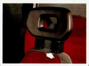
To raise or lower the restraint, push in the release while you pull up or push down on the restraint.
