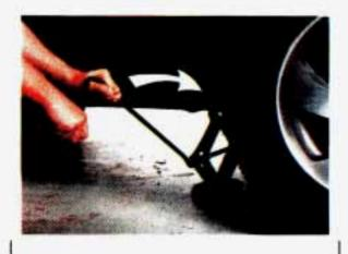
Raise the vehicle by rotating the wheel wrench clockwise. Raise the vehicle far enough so there is enough room for the spare tire to fit.
