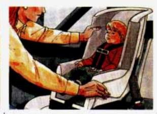
Pull the rest of the shoulder belt all the way out of the retractor to set the lock. To tighten the belt, feed the shoulder belt into the retractor while you push down on the child restraint. Push and pull the child restraint in different directions to be sure it is secure.
