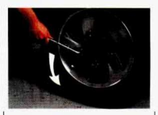
Insert your key into the wheel lock and pull the wheel lock off.
