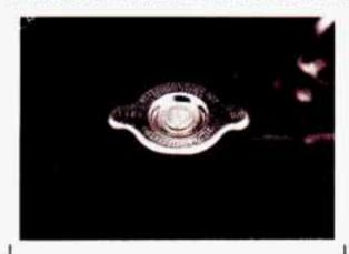
Then replace the pressure cap. Be sure the ears on the pressure cap line up like this.
